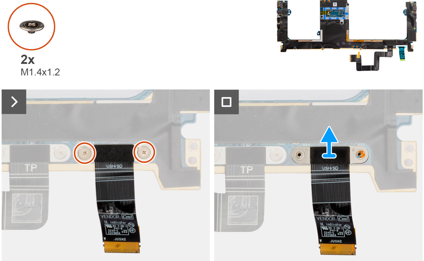
Figure 18. Removing the USH and SD card reader daughterboard FPC
