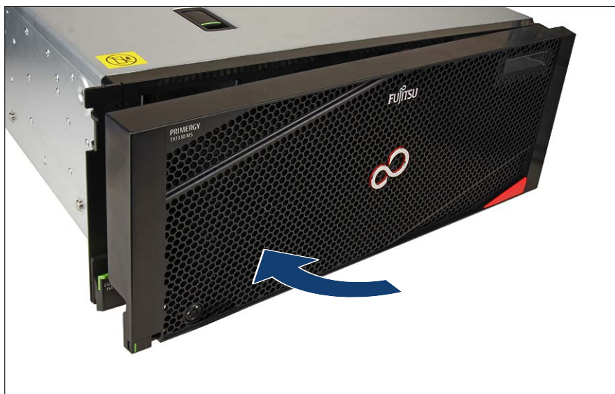
Figure 22: Installing the front cover
