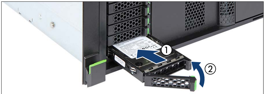
Figure 34: Installing the 2.5-inch HDD/SSD module
