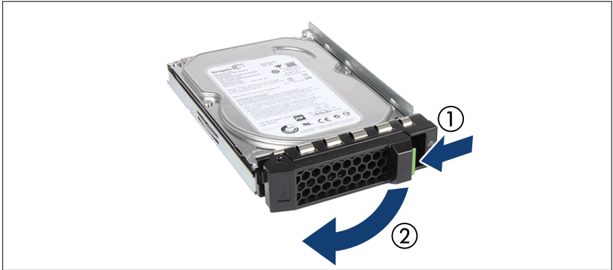
Figure 30: Opening the locking lever
