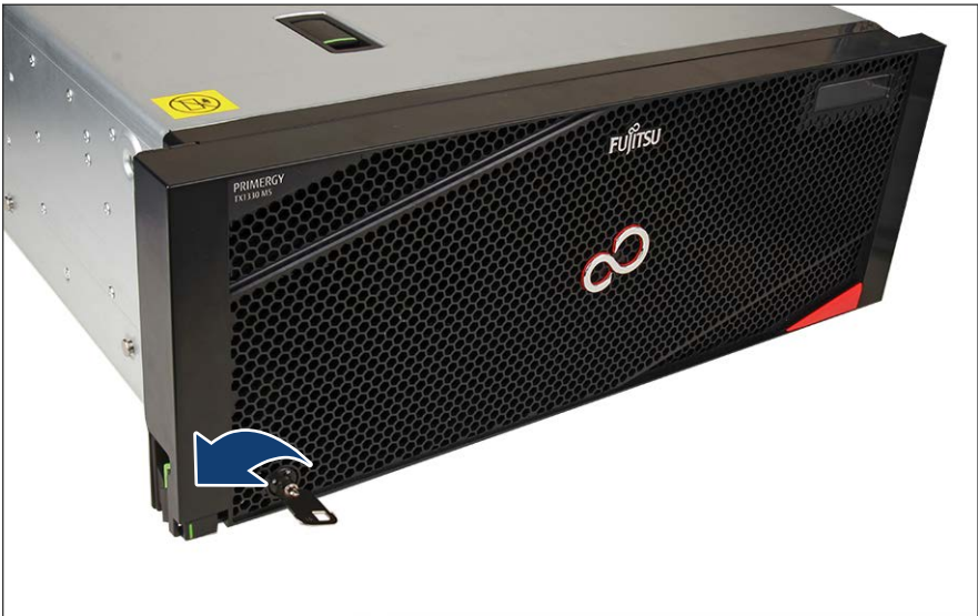
Figure 24: Turning the key
