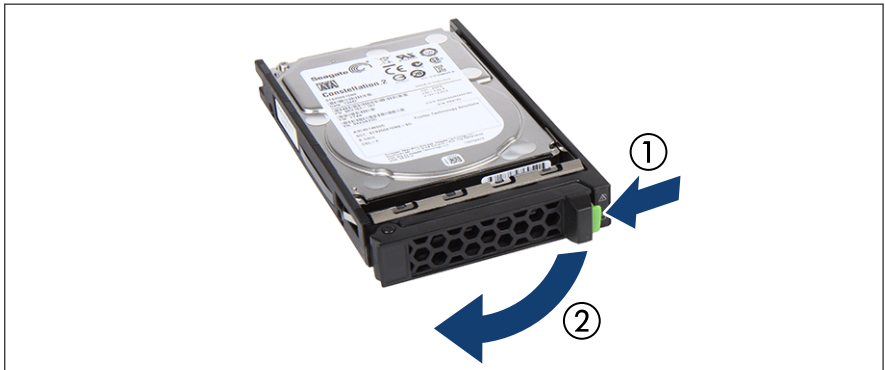
Figure 33: Opening the locking lever
