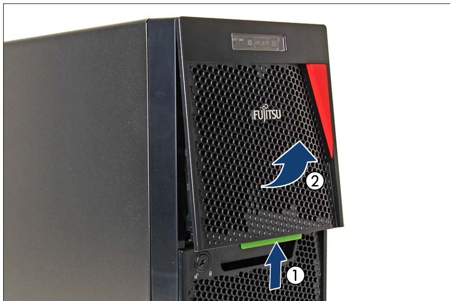
Figure 27: Removing the accessible drive bay cover
