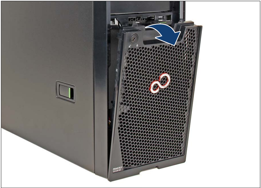
Figure 28: Removing the HDD bay cover
