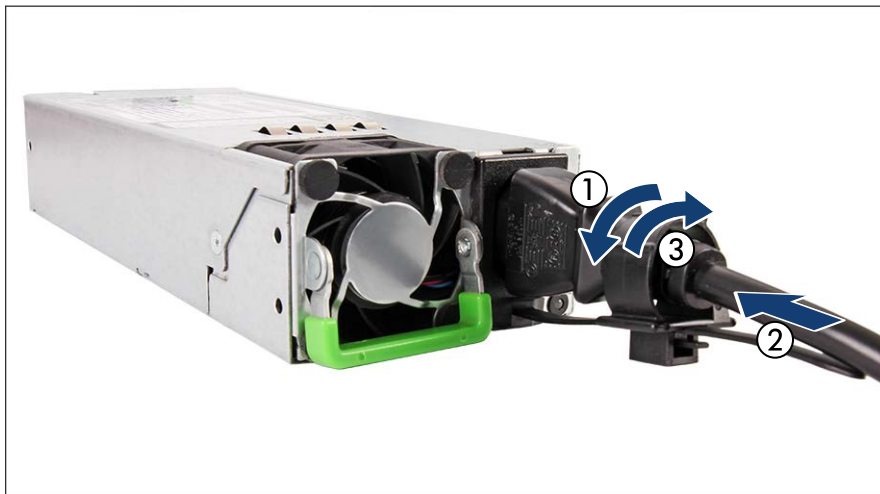
Figure 26: Locking the cable clamp of a PSU
