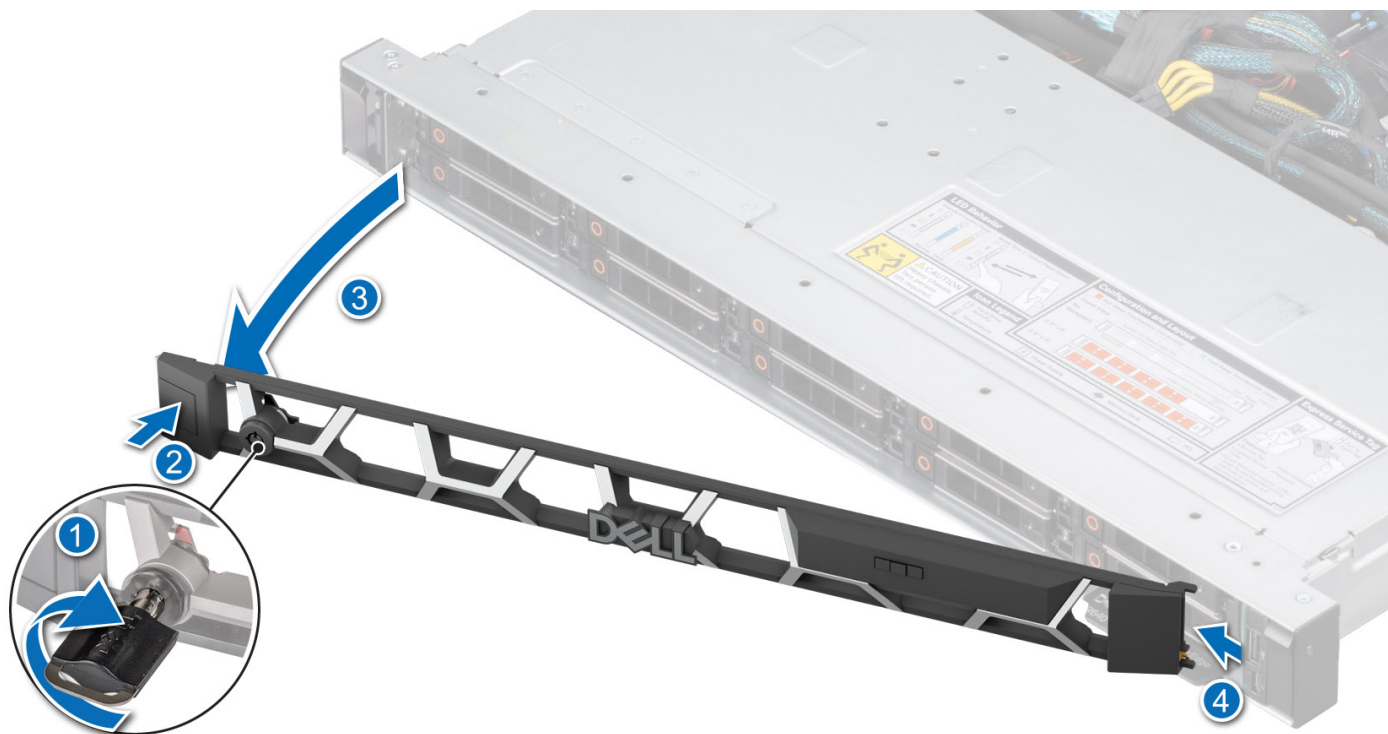
Figure 22. Removing the front bezel with the LCD panel
