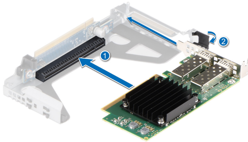
Figure 99. Installing an expansion card into a Riser 1a
