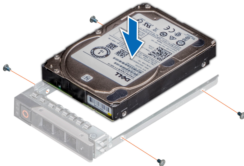
Figure 39. Installing a drive into the drive carrier
